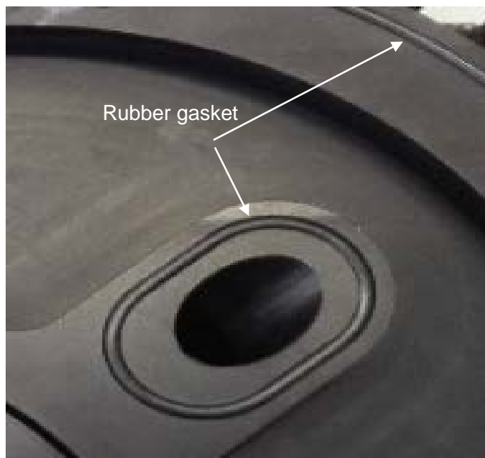
Figure 16. It is important that the rubber gaskets shown in the picture are correctly placed. These gaskets are present in both filter changer layers.
