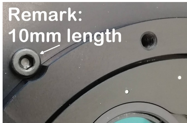
Figure 15. Short screw must be placed in the middle.
