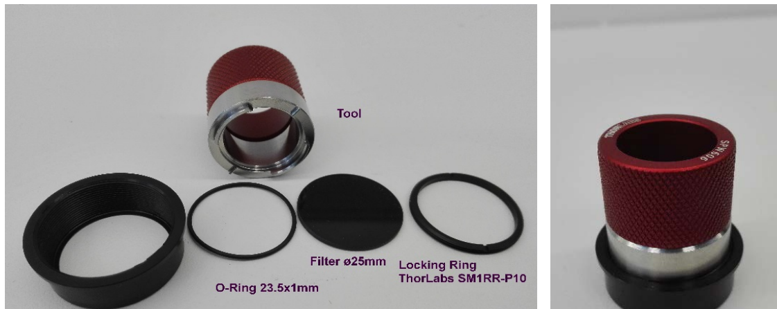
Figure 29. Individual items in the filter assembly (left) as well as the tool used for tightening the locking ring (right).
