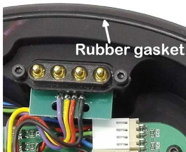
Figure 14. Rubber gasket in the base unit.
