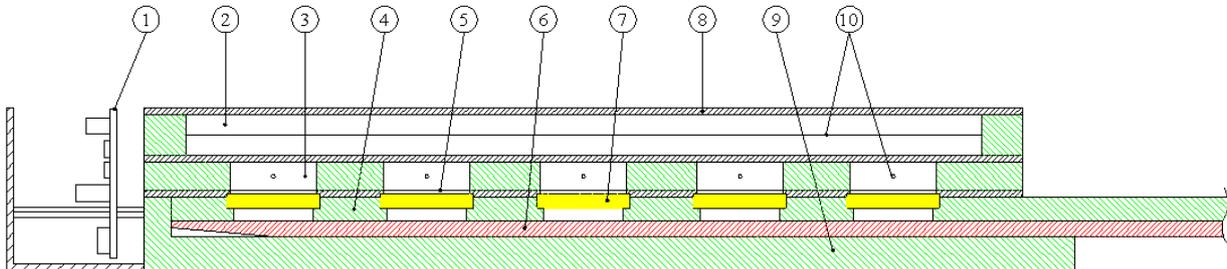
**Fig. 1** The five-sample beta GM multicounter, schematically.
