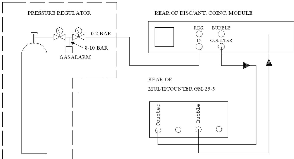
Fig. 4. Flow diagram of the counter gas connections to the multicounter GM-25-5. The pressure from the cylinder is reduced to 0.2 bar and the gas flow is adjusted with the flow regulator (reg.) to approx. 100-120 bubbles per min. (NB! Counters bought before 1. august 2010 have a different type of bubble chamber that should be set to 50-60 bubbles / min.). Note that the gas is led through the guard counter first and then through the sample counters.
