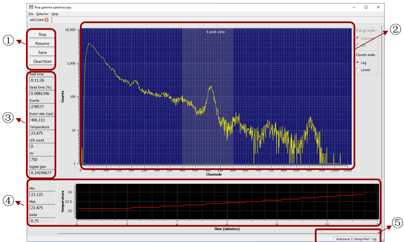
Fig. 1.4: Graphic User Interface of GammaAcq software. ① command buttons, ② gamma spectrum histogram, ③ counting/setting parameters, ④ temperature of the detector, and ⑤ information bar.
