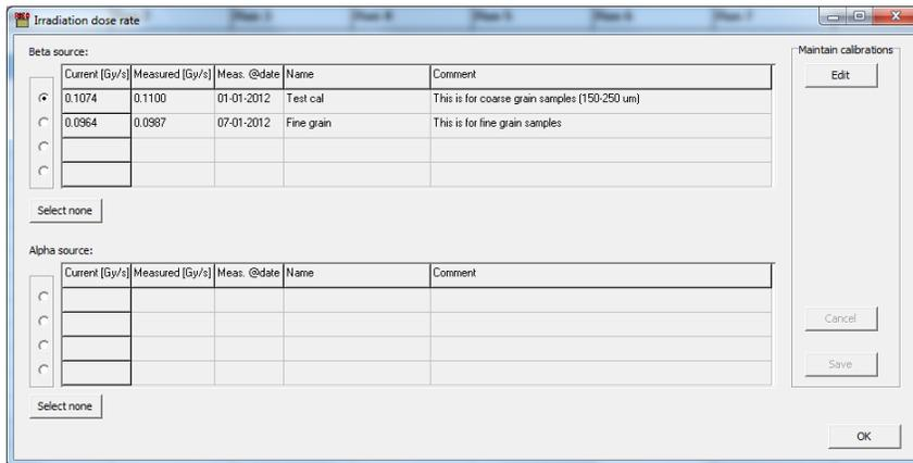
In the form you may select a beta- and/or alpha- dose rate calibration. When a measurement is done, the current dose rate and associated dose rate error, i.e. measured dose rate and dose rate error corrected for radioactive decay, is stored with the data in the bin-file. This enables Analyst to make a conversion of estimated dose from *equivalent seconds* (s) to *Grays* (Gy).
