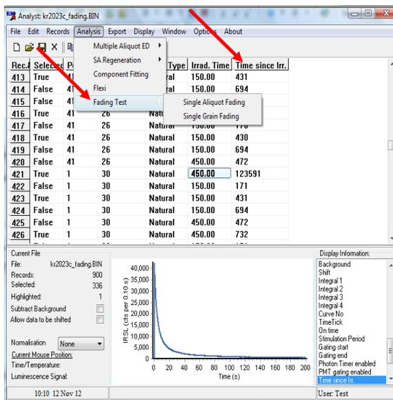
The time between start of irradiation and start of measurement is automatically recorded in the bin-file. This time is compensated for the duration of the irradiation to give  $t^*$  (Aitken (1985), Appendix F, p. 280)
