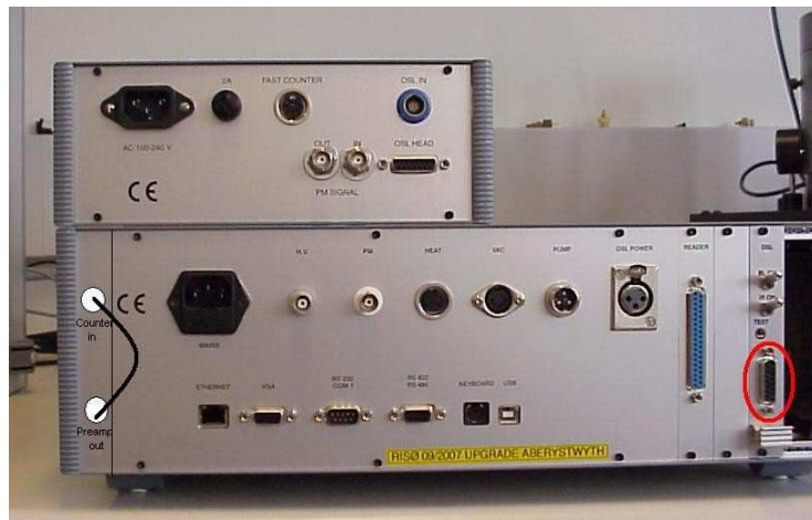
Figure 9: Running the system in true CW mode (Controller based system).
