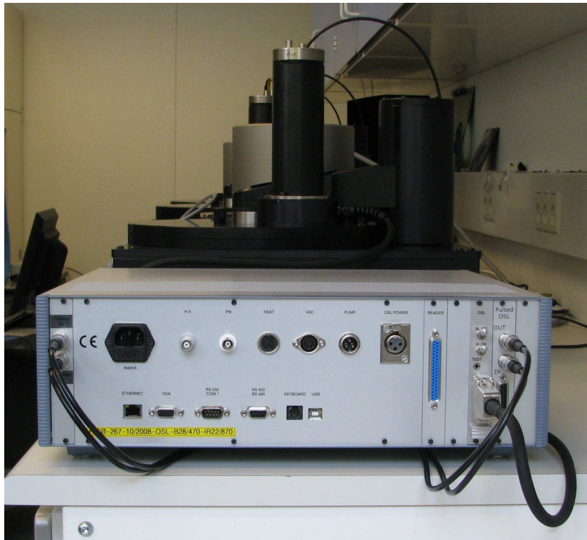
Figure 10: Photo showing the connections on the back of the controller.
