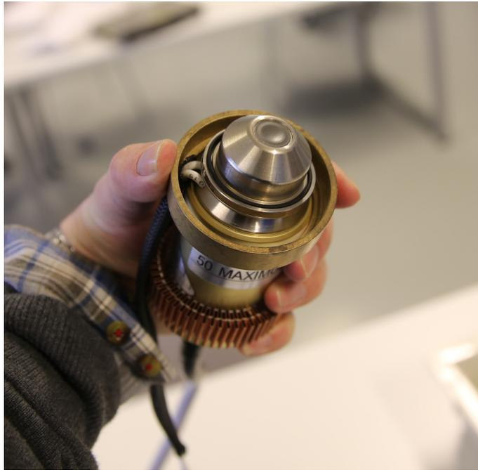
Figure 2.1: The Varian VF-50 X-ray tube before assembly.
