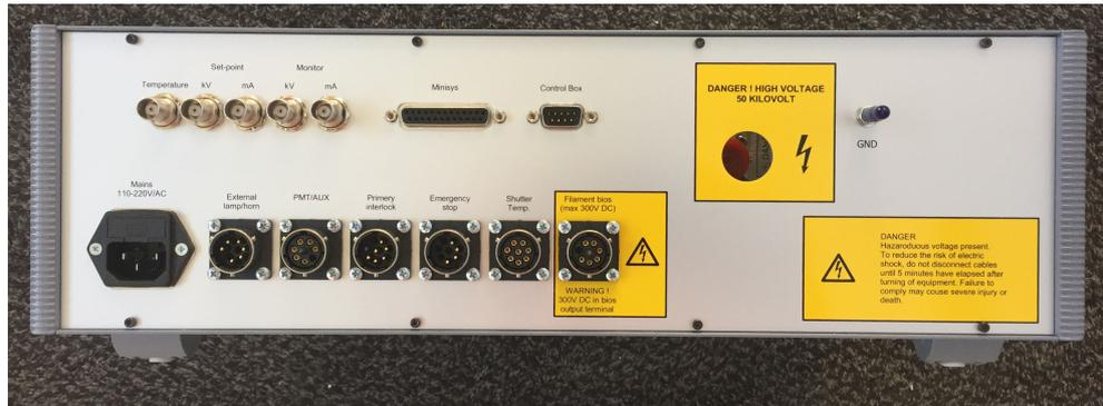
Figure 2.12: Labels on the back of the XHV-1 control unit.
