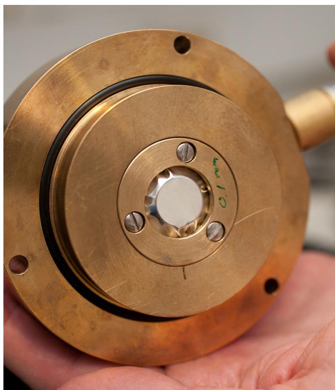
Figure 2.8: The x-ray collimator window.
