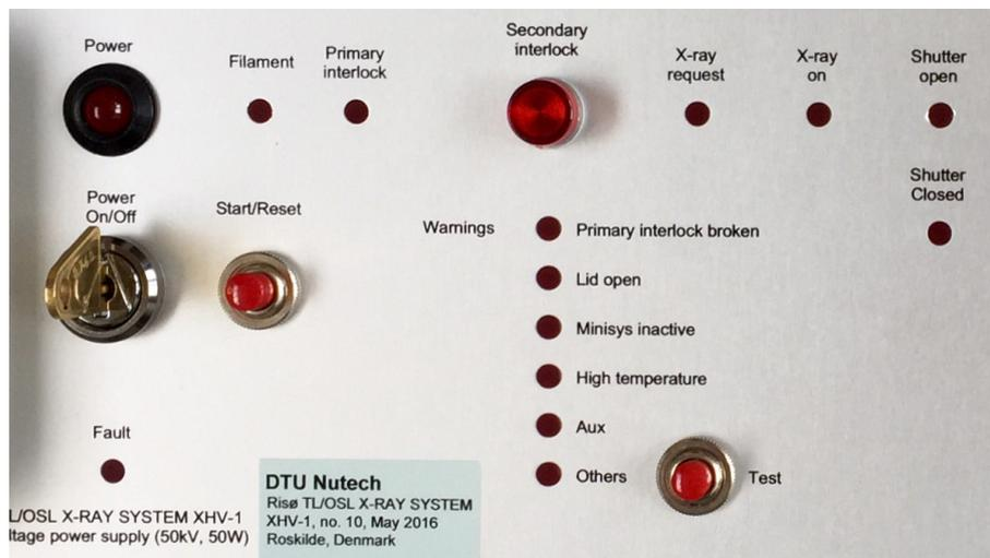
Figure 2.6: Indicators with status information on the front of the XHV-1 control box.
