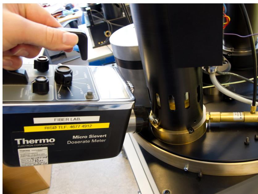
Figure 2.3: The x-ray tube during leakage testing.
