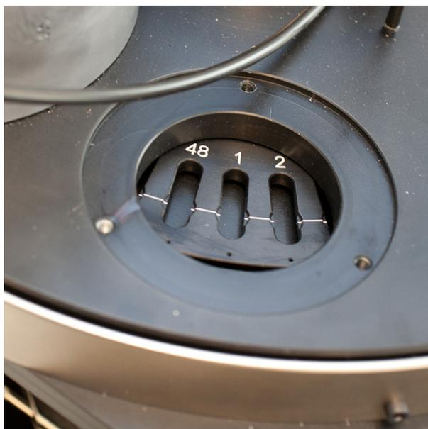
Figure 2.9: The x-ray tube is mounted at this position.
