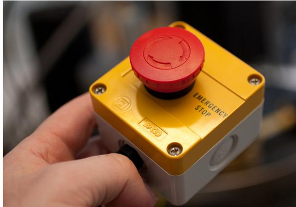
Figure 2.4: The x-ray emergency stop.
