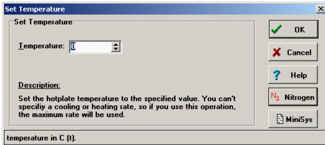
Set the hotplate to the desired temperature. If the desired temperature is higher than the current temperature then the hotplate is heated at the maximum temperature. If the desired temperature is below the current temperature then the set point is changed instantly in order to achieve a maximum cooling rate.
