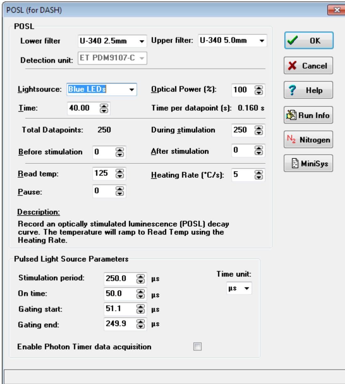
Define parameters for recording a Pulsed Optically Stimulated Luminescence (OSL) decay curve. To measure Phosphorescence decay, select “none” as the light source.
