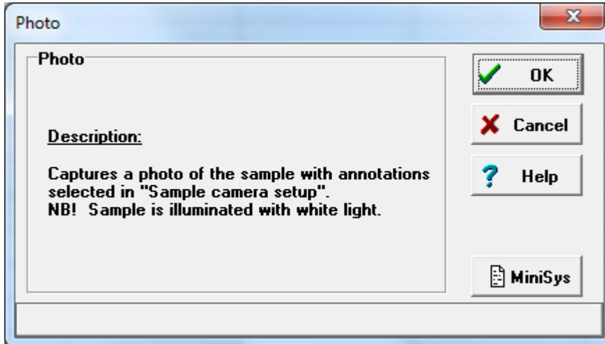
Uses the sample camera to produce a photo of a sample. The photo is stored in a directory with the name of the bin-file, and the name of the picture file is *<bin-file name>\_rrsspp.jpg*, where rr is run no., ss is set no., and pp is position no.
