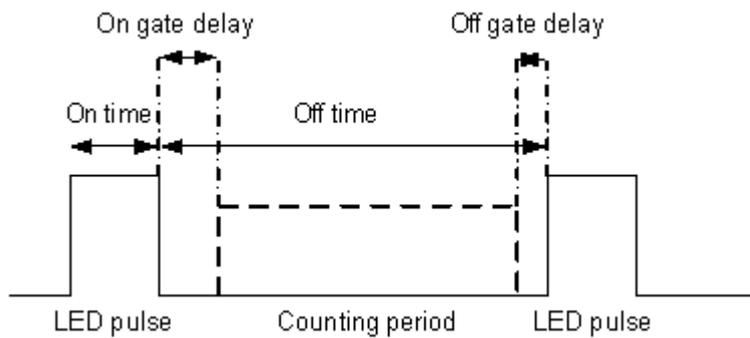
If **Gate PMT to count only in off period** is checked, counting is only done in the interval marked “counting period” in the above figure.
