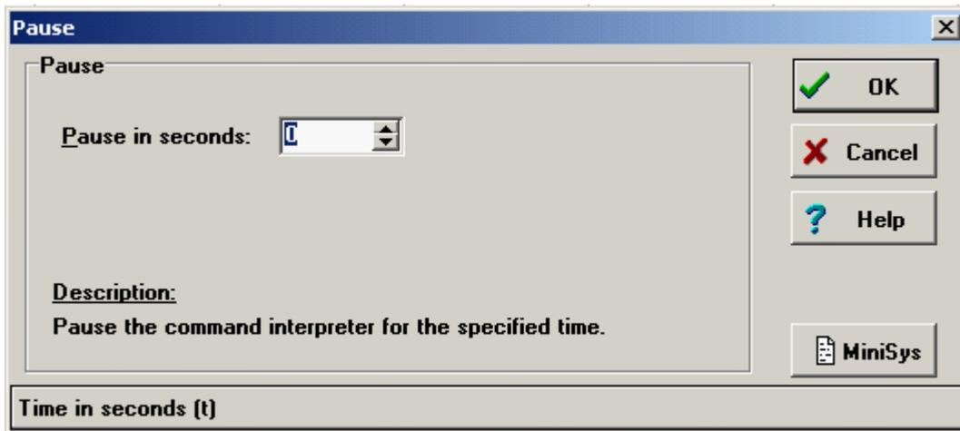
Pause the Mini-Sys command interpreter for the specified time. During a pause both the Command running status bit and the Command interpreter paused status bit are set to true (see Mini-Sys documentation for a description of all status bits).
