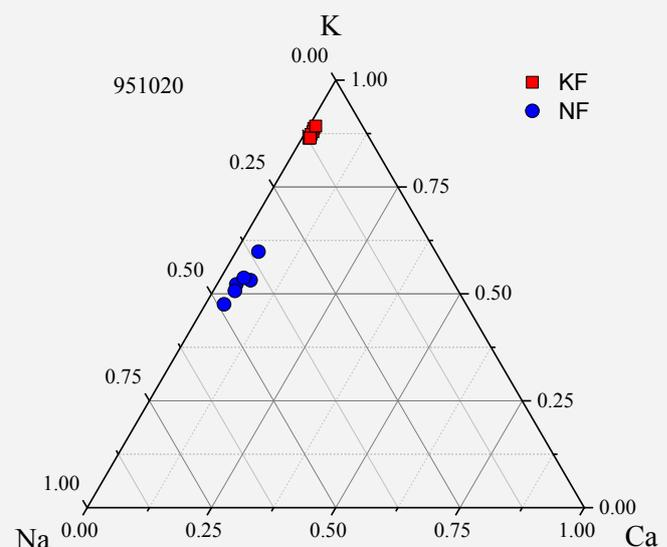
Ternary diagram showing the results for K-feldspar rich ( $\rho < 2.58 \text{ g cm}^{-3}$ ) and Na-rich extracts ( $2.58 \text{ g cm}^{-3} < \rho < 2.63 \text{ g cm}^{-3}$ ) measured with the Risø XRF-attachment. Six multi-grain aliquots were measured per extract. The 180-250 μm feldspar grains were extracted using conventional sample preparation techniques (HCl, H<sub>2</sub>O<sub>2</sub>, HF, heavy liquids) from sediment from Greenland.
