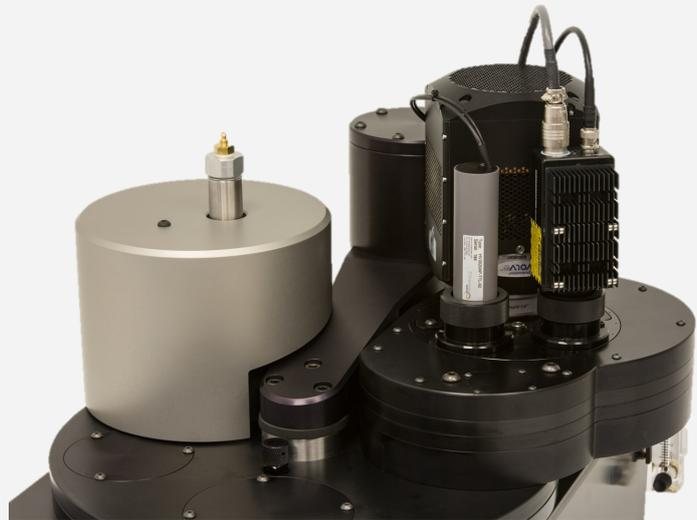
DASH shown with detector changer and mounted with the standard PMT (item 2001), a red PMT (item 2002) and the EMCCD camera (item 2004)
