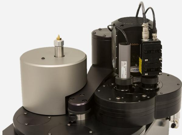
The detector changer is the top layer of the Detection and Stimulation Head (DASH) shown to the right. Here the detector changer is equipped with a standard blue/UV PMT (item 2001), the red sensitive H7421-40 PMT (item 2002) and the EMCCD camera (item 2004).
