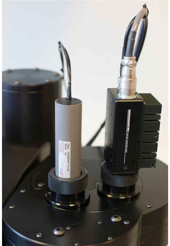
The UV/Blue sensitive PMT (item 2001) mounted for with the red sensitive PMT detection module (item 2002). The detector changer (item 1003) is a prerequisite when several detectors are mounted simultaneously.
