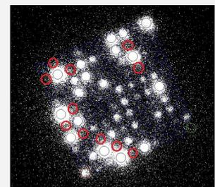
Standard single grain discs with depth and diameter of 300  $\mu\text{m}$ . Picture on the right shows blue stimulated quartz OSL recorded with the EMCCD option (item 2004; Thomsen et al., 2015).
