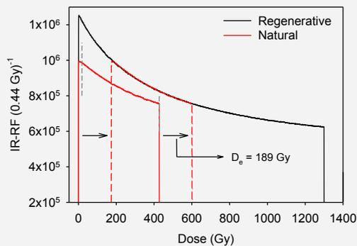
Principle of a fit of the additive dose response curve (solid red curve) onto the regenerative dose response curve (black) using *RLanalyse*; the horizontal displacement gives the  $D_e$  value. The vertical dashed grey lines indicate the region of the additive dose curve that was used for the fit. The best fit is shown using a dashed red line. (Buylaert et al., 2012)
