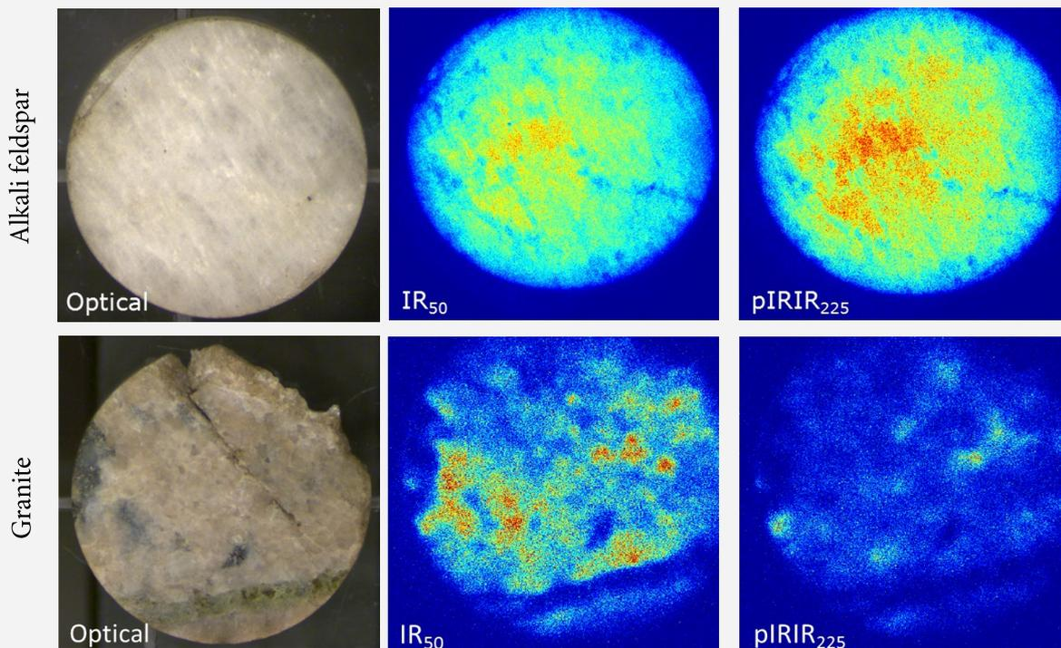
Optical and EMCCD images of rock slices of alkali feldspar and granite measured using BG3 and BG39. The luminescence images were obtained after a dose of ~120 Gy and summation of the first 4 s of IRSL.
