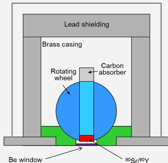
Schematic diagram of the cross section of the beta irradiator. The  $^{90}\text{Sr}/^{90}\text{Y}$  source is placed in a rotating aluminium wheel, which is pneumatically activated. The source is shown in the *on* (irradiating) position. When the source is *off* the wheel is rotated 180°, so that the source points directly at the carbon absorber. Redrawn from Markey et al. (1997).
