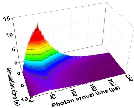
TR-POSL surface plot of a quartz sample with on-/off-time of 50/200  $\mu\text{s}$ .
