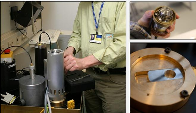
Left: The X-ray tube during testing at DTU Nutech. Top: The Varian VF-50 X-ray tube before assembly. Bottom: The X-ray collimator block with mechanical shutter.
