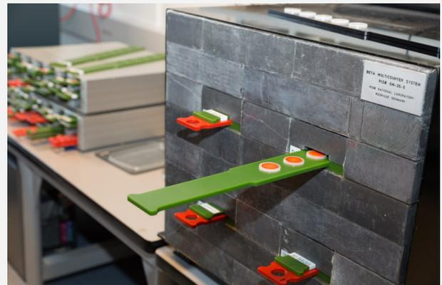
Beta counter is mounted in a lead castle. A sample slide is partially inserted into the counter.
