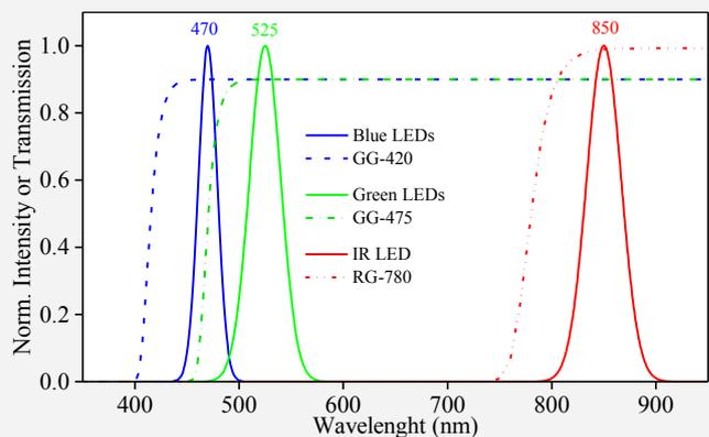
Emission characteristics of the stimulation LEDs and transmission characteristics of the long-pass filters used in front of the individual LEDs.
