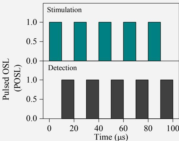
Schematic drawing showing stimulation and detection timing for on/off times of 10/10 μs.
