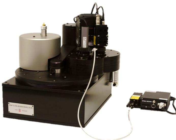
Example of how a user-supplied external light source can be coupled to the Reader using the empty position in the DASH.
