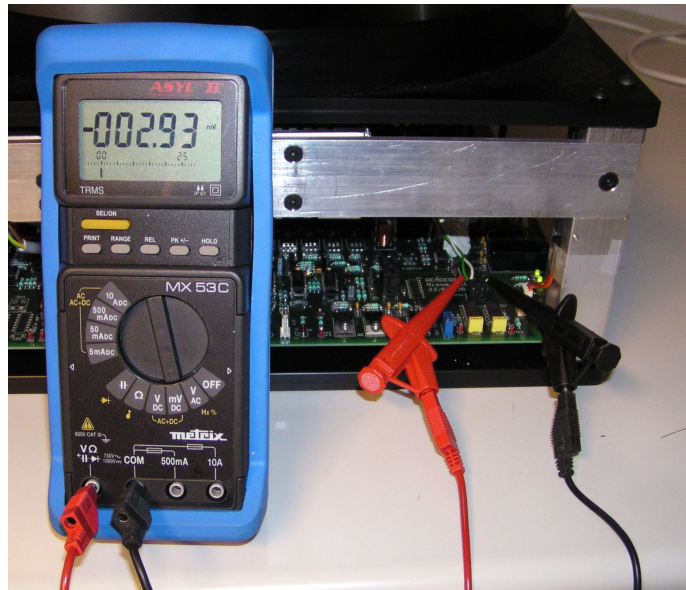
Figure 1: Reading the thermocouple voltage (range 100 mV max)
